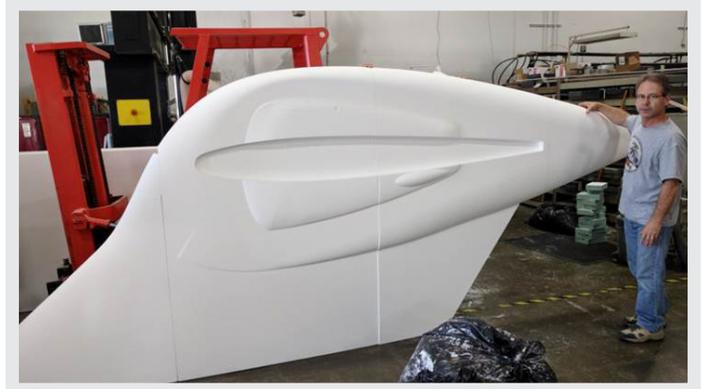
(Above) Using PacMin Studio's large format CNC machine, the team cut the massive Challenger 350 in just 7 days.
