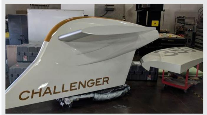
(Above) Even though the tail was produced from lightweight materials, it still weighed over 200 pounds. In order to support the tail's weight and height, the tail is reinforced with an adjustable steel structure and base.
