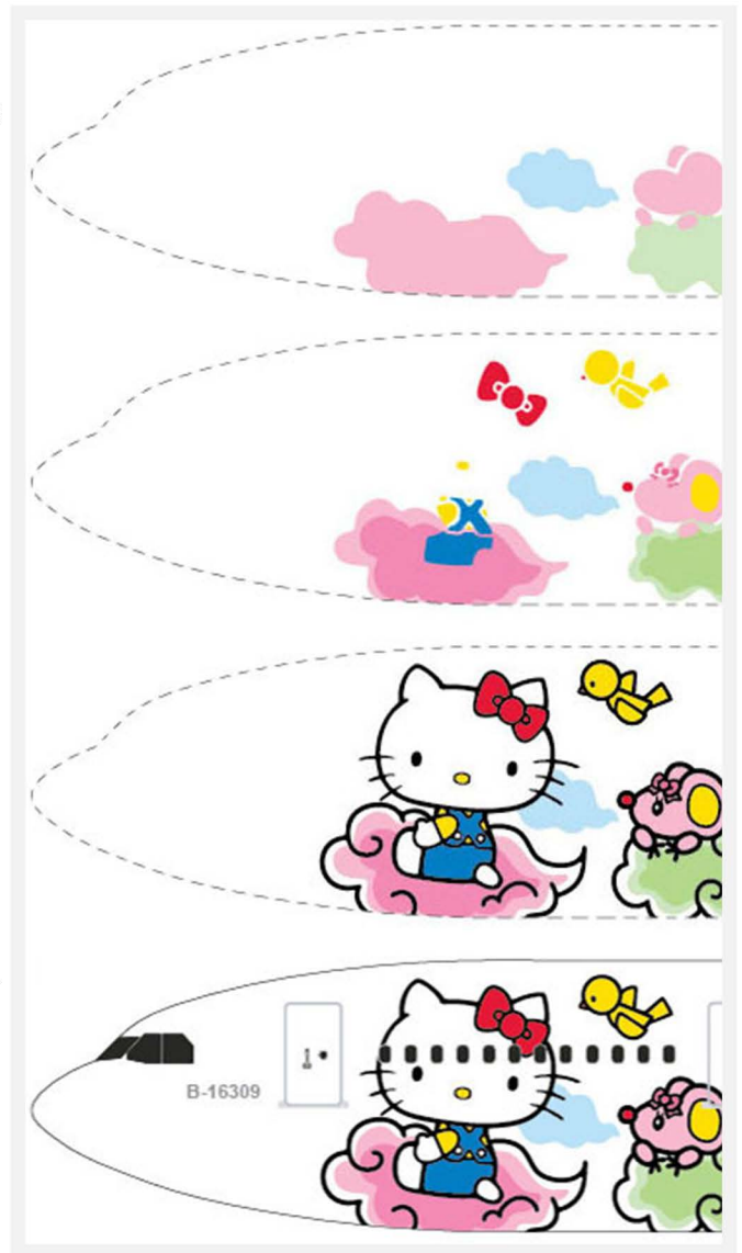
(Above) Computer mock-up of printing process. Each color is printed one at a time to improve accuracy and registration (airplane accents, such as the windows and doors, are also printed separately). The entire printing process took approximately 40 hours.
